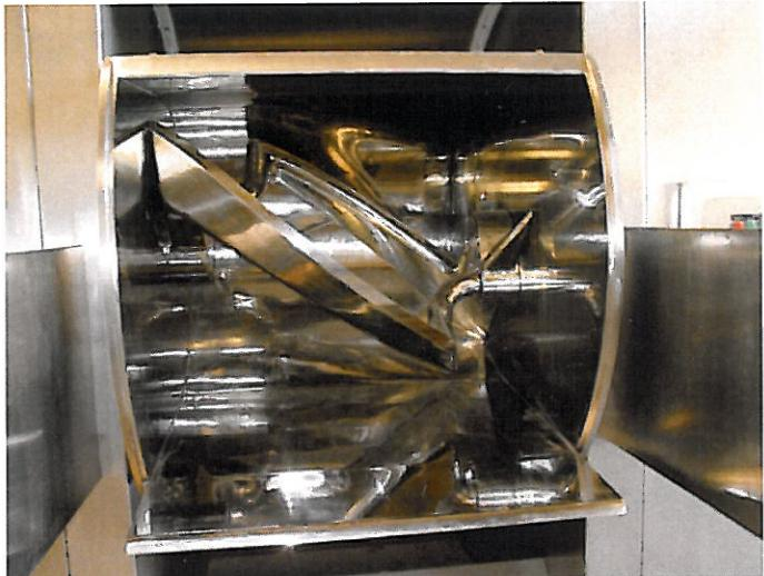
The same can bend of 105 ° thanks to a hydraulic system that allows an easy and convenient emptying.
